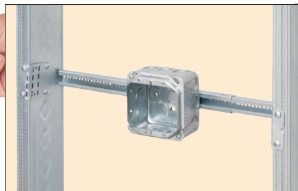
Mount SliderBar on studs with #8 x 1/2" screws. Position box on bar. Tighten screws inside box.
